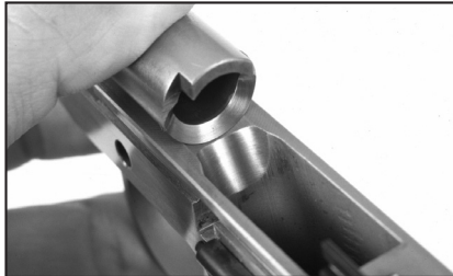
Reliability of the Springfield, Inc., Trophy Match pistols is enhanced by the polished feed ramp and generously throated barrel.
